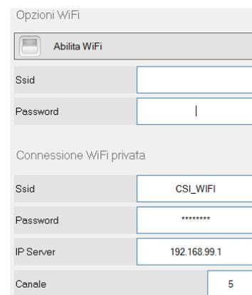
The screenshot shows a configuration window titled "Opzioni WiFi". It contains a toggle switch for "Abilita WiFi" which is turned on. Below this are two sections: "Ssid" and "Password" with empty input fields. A second section, "Connessione WiFi privata", contains four fields: "Ssid" with the value "CSI\_WIFI", "Password" with "\*\*\*\*\*", "IP Server" with "192.168.99.1", and "Canale" with "5".
